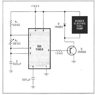
**Adjustable-speed pump driver.** This IC timer arrangement drives the Bendix plunger-type electric fuel pump at a rate of 16 strokes per second. Adjustment of R<sub>2</sub> permits other pumping rates.
